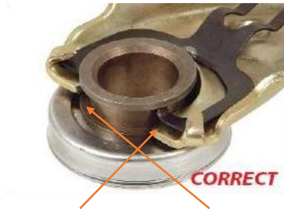
Retaining clip on the inside of bearing
