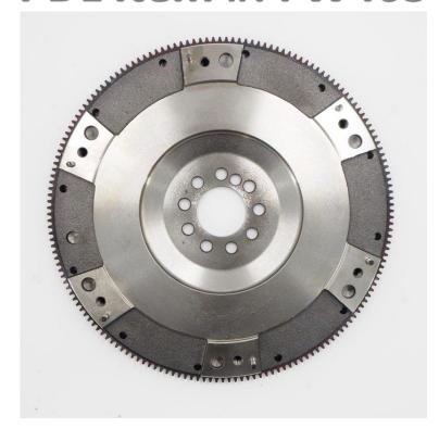
This Flywheel is for use in 2011 and 2013 Chevrolet Corvette 6.2L ZR1 applications. The flywheel is an integral part of clutch replacement. It must provide a smooth, flat surface for proper clutch operation.
