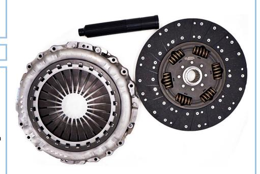
This is a new Clutch Kit for use with Volvo I-Shift and Mack mDrive automated manual transmissions which engages and disengages without the use of a traditional in-cab clutch pedal.
